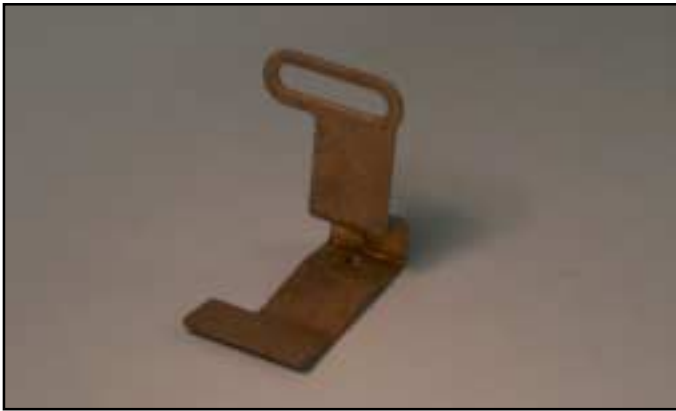
Fig. 38 Original Trip Finger Removed from an Electrically Operated Breaker with Short Trip Shaft.
