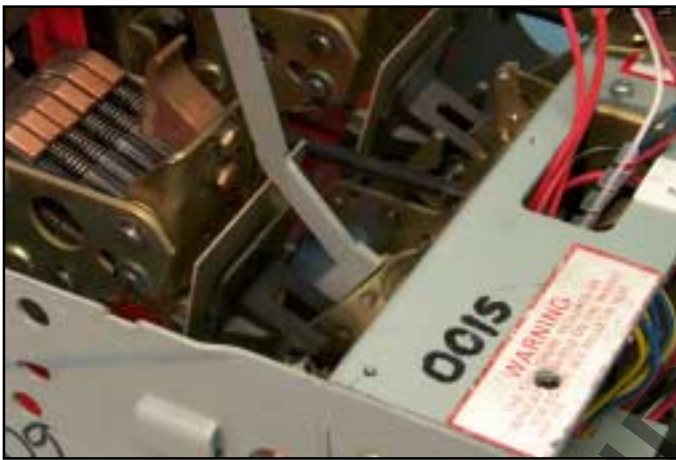
Fig. 45 Slow Close Handle Engaged in the Closing Link.
