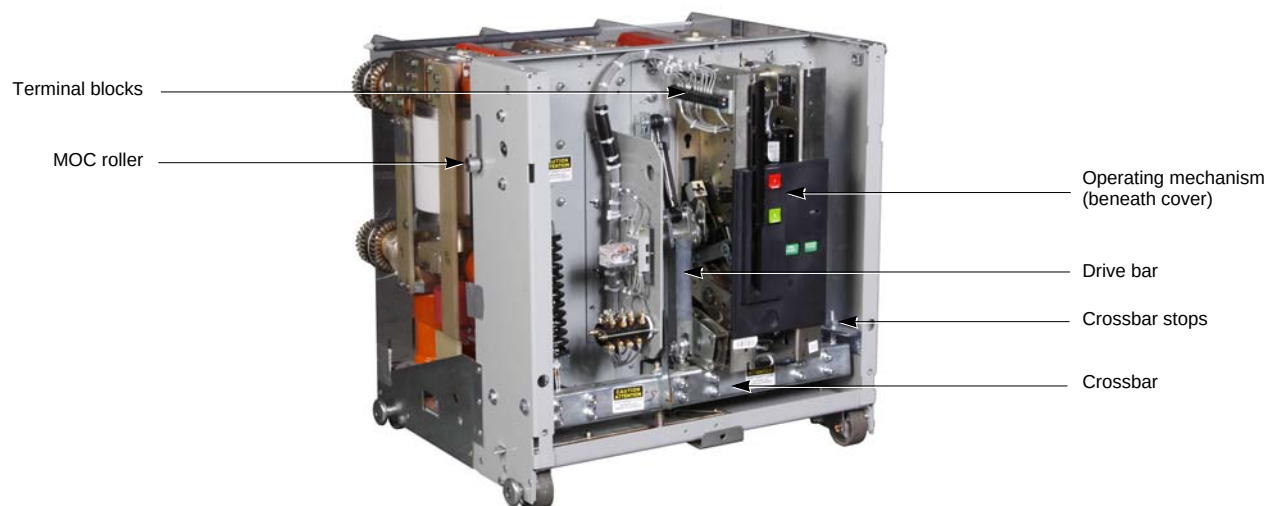
Figure 5: Circuit Breaker—Left Front View with Cover Removed
