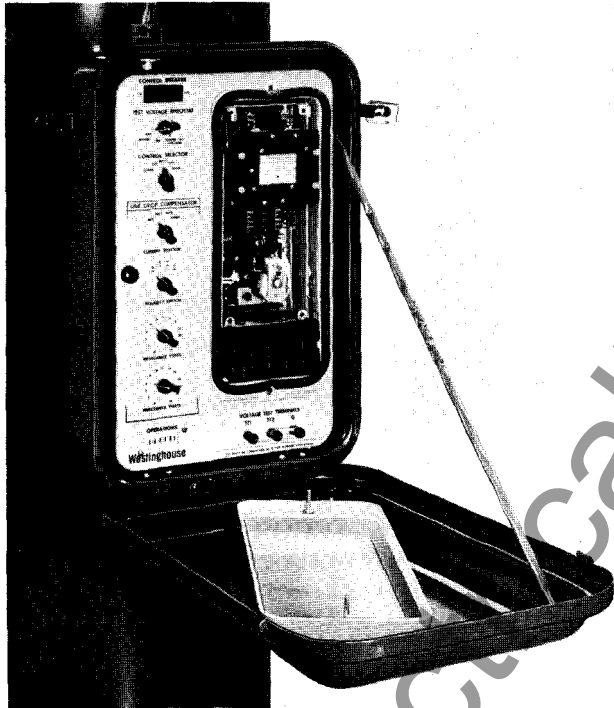
Fig. 2 - Regulator Control Panel with Cover Removed from CVR Relay
