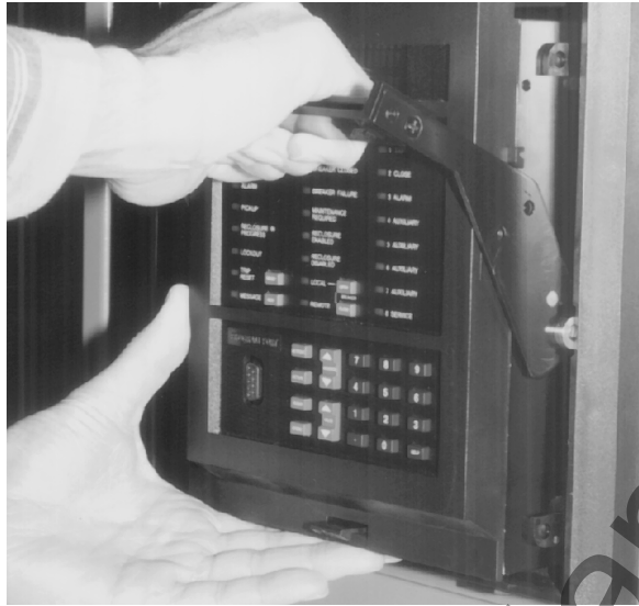
Figure 3-7: SLIDING THE UNIT OUT OF THE CASE
