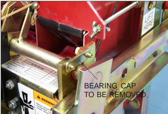
Fig. 55 Bearing Cap to be Removed (LAF-1600 C).
