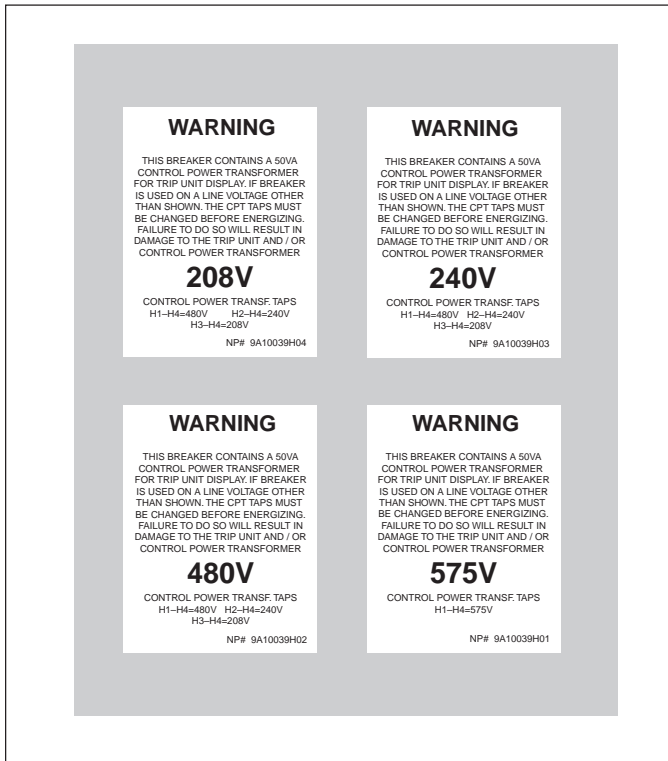
Fig. 72 CPT Voltage Labels Supplied with the CPT Kit.
