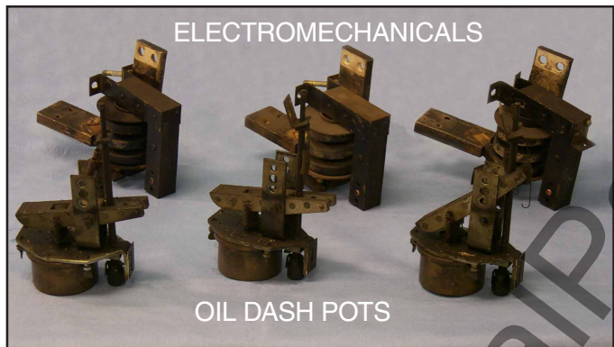
Fig. 1 Overview: Original Components Removed from the Breaker.
