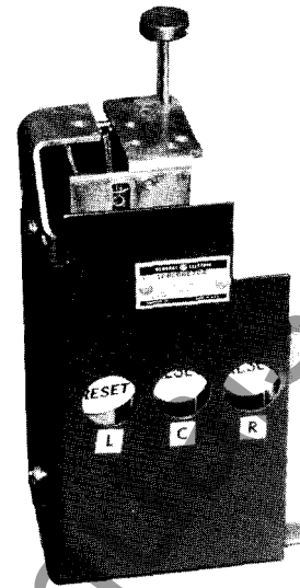
Figure 4. Open Fuse Lock-out
