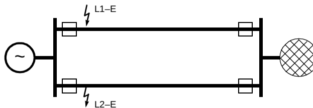
Figure 6-14 Multiple fault on a double-circuit line next to a generator
