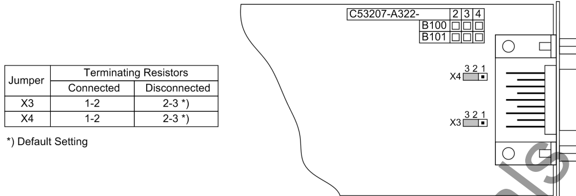
Figure 3-9 Position of the plug-in jumpers for configuration of terminating resistors of the Profibus interface
