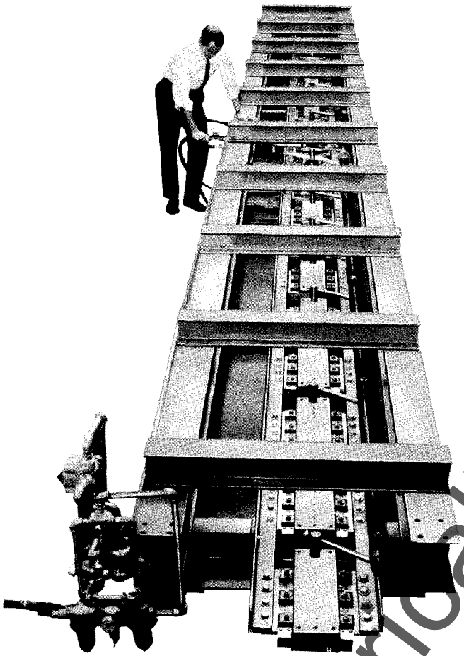
140,000 Ampere 4.5 Volts dc Cell Shorting Switch Designed for the Chlor-alkali Industry
