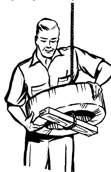
Fig. 2. Suggested method of handling CT. Place crossbar under spacers when provided
