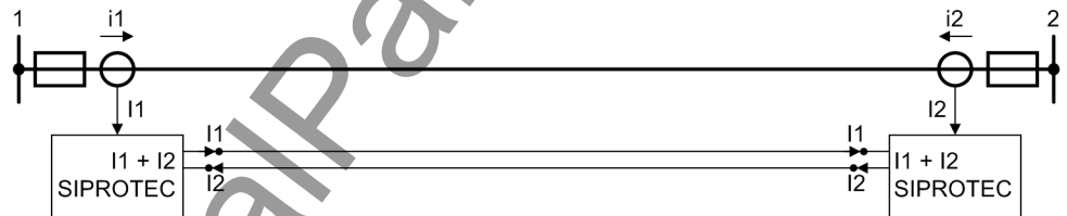
Figure 2-24 Differential protection for a line with two ends
