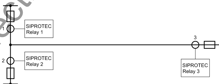
Figure 2-1 Protected object with 3 ends and 3 devices
